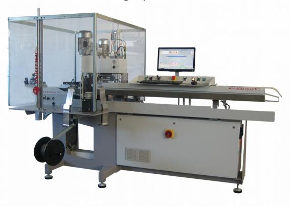
AM350 quattro is the fully automatic machine projected for processing the flat and nily cable. It's a machine very easy to use and with change set up very fast. As AM300 quattro require a low maintenance and easy to use.
