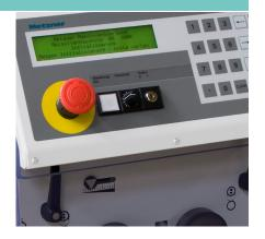
machines. The basic version of the AM 2000 already supports the connection of marking and labelling devices, as well as the control with a PC/laptop for machining complex batches in cable assembly.
