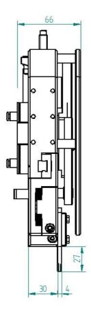
Picture: Dimension welding-pincer SZ-2030 with pneumatic drive, without mounted attachments
