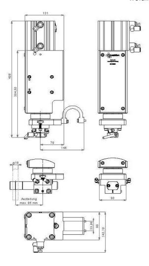
Picture: Dimension welding head SK-2350 without fixing/ mountings
