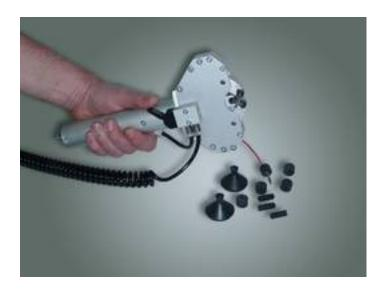
Commercial description for this type of tool: **EXPANSORA MINI.**With an air pressure of 5 bar the pneumatic device is ready for operating.
