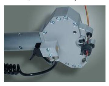
The cable or hose is easy to put through the widened opening.
