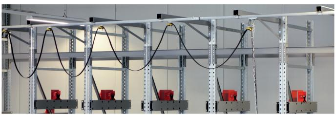
Cable trailing system for rack mounting
