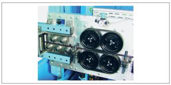
Fig. 2 MESSBOI BELT installed in a machine with roller cages and straightening
