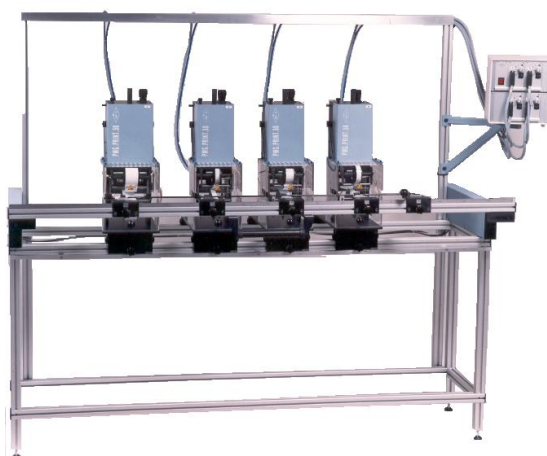
Multi head device with inserting carriage for ring and text printing
